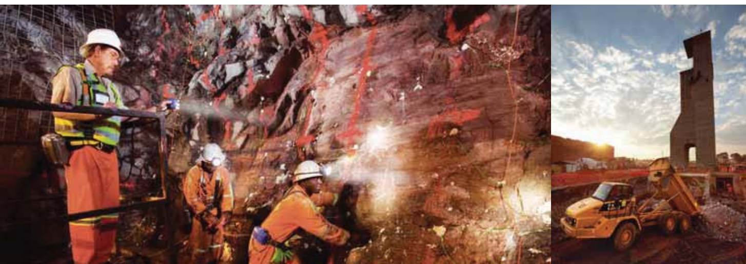
Charging-up operations in the East Limb conveyor access decline at the Konkola North Copper Mine
