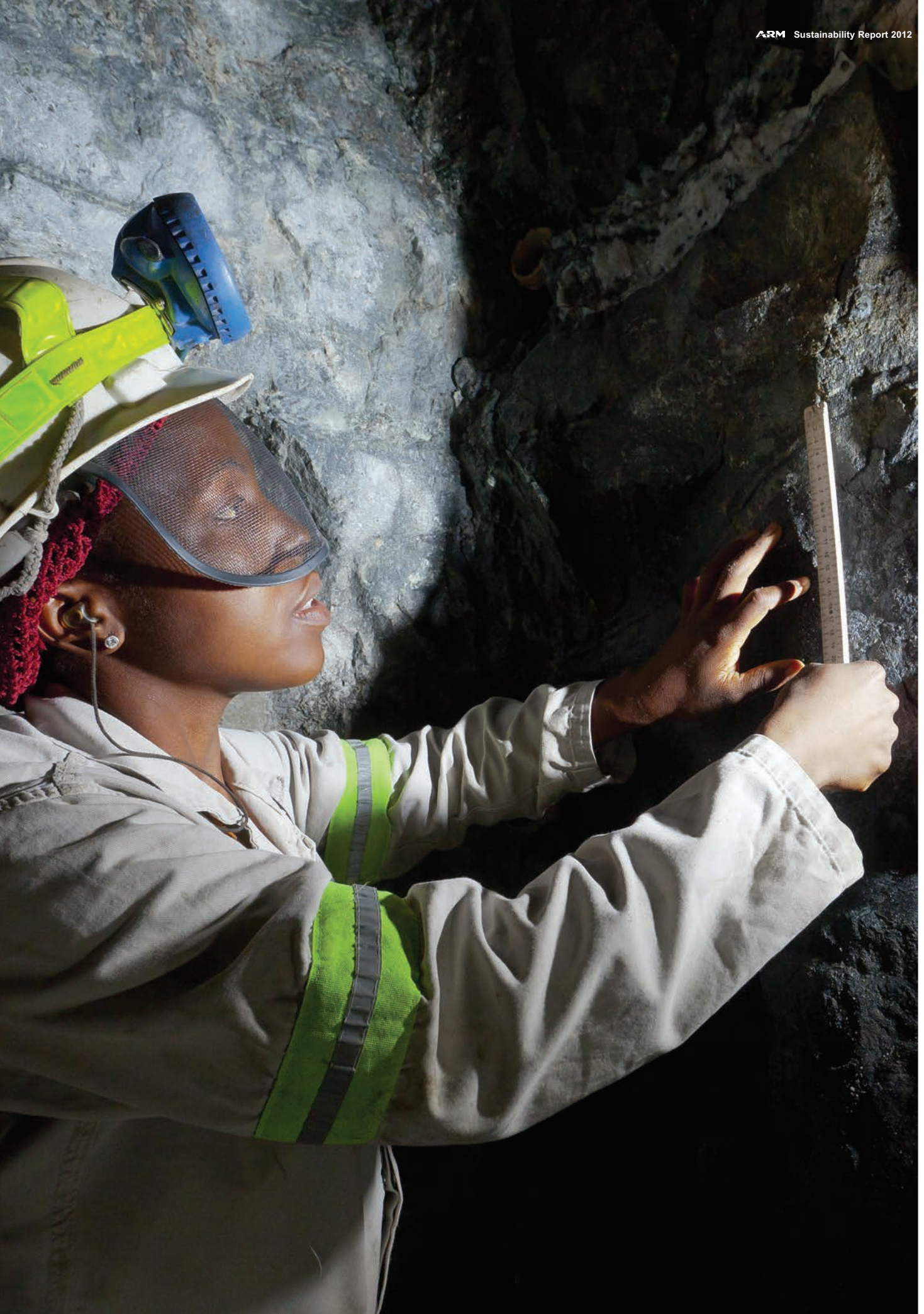
Rita Nkambule, Grade Controller, measuring stope width at Modikwa Platinum Mine
