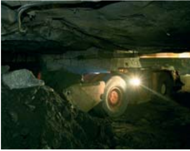
Load Haul Dump (LHD) operation
