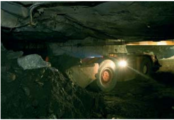
Load Haul Dump (LHD) operation
