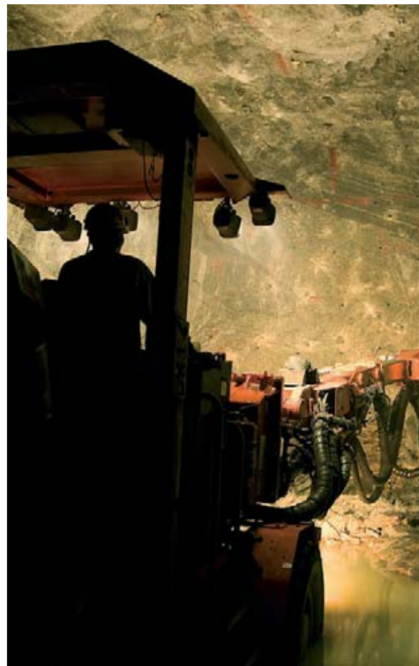
Twin boom drill rig
