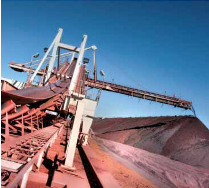
Stockpiling of iron ore prior to railing at Khumani Iron Ore Mine
