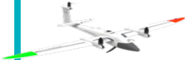
The Trinity F90+ drone used to inspect tailings dams at Impala Rustenburg.
