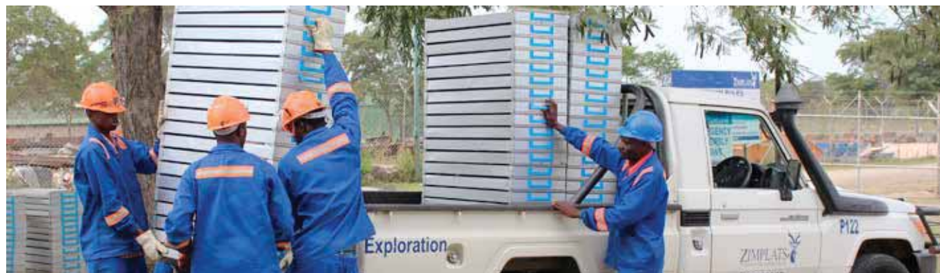
Receiving core trays for exploration drilling, Zimplats.
