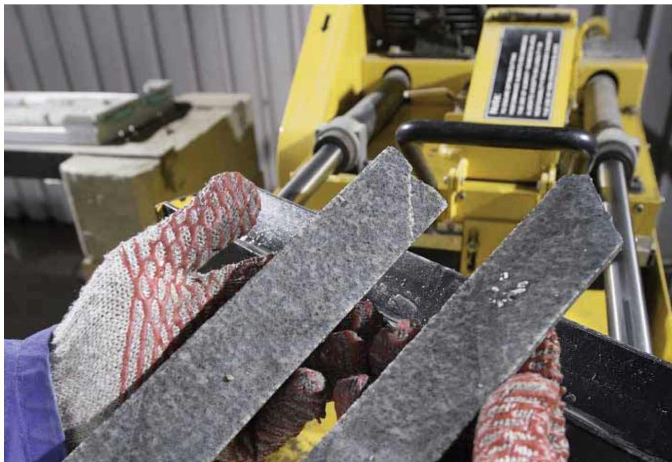
Splitting of borehole core.
