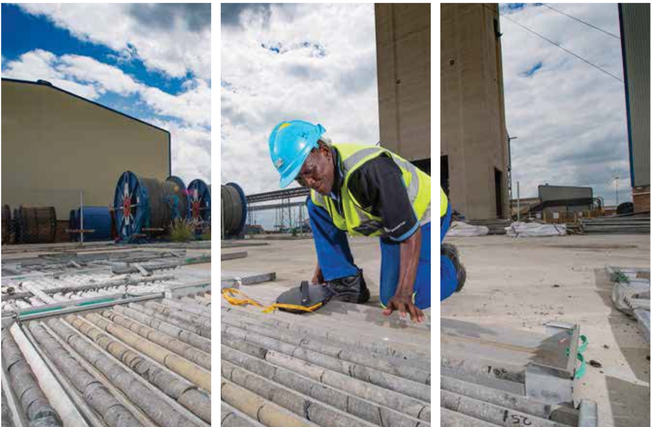
Measuring drilled underground core at 16 Shaft, Impala
