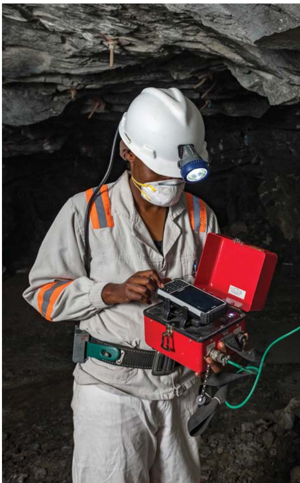
Measuring stress variations in underground pillars at Zimplats
