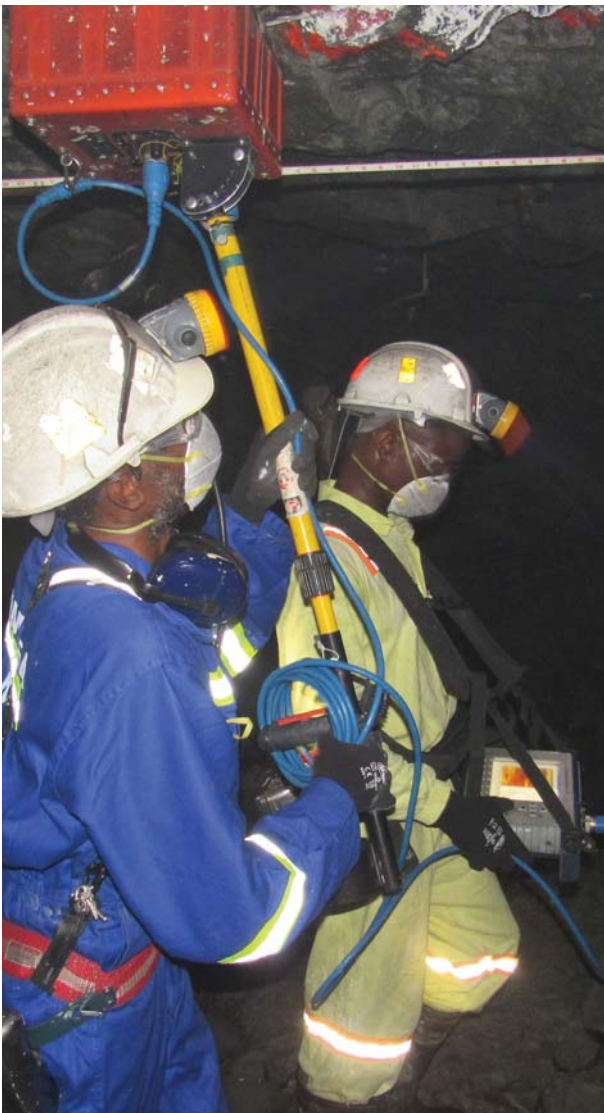
Ground penetrating radar survey
