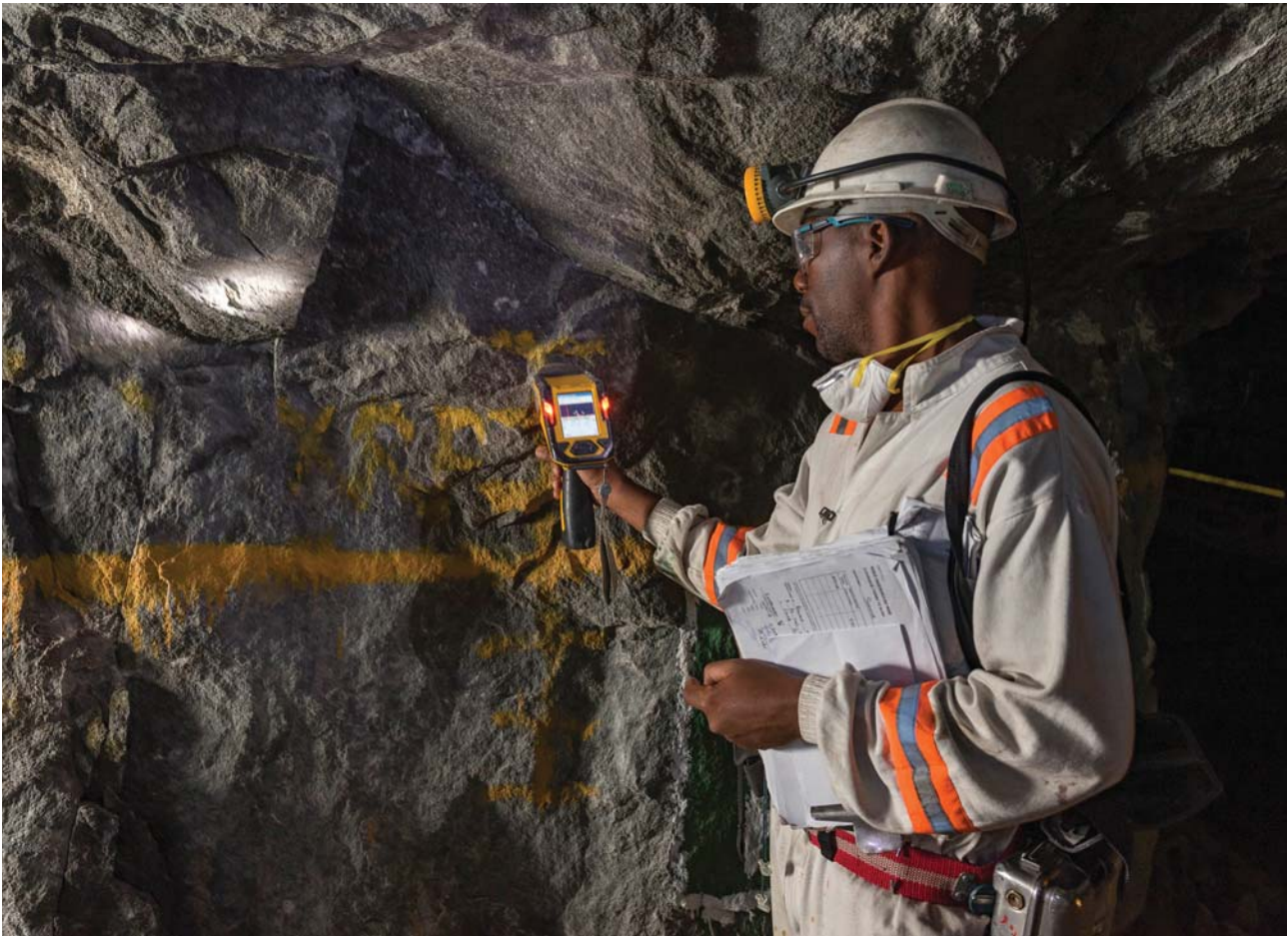
Grade control by means of XRF scanning at Zimplats
