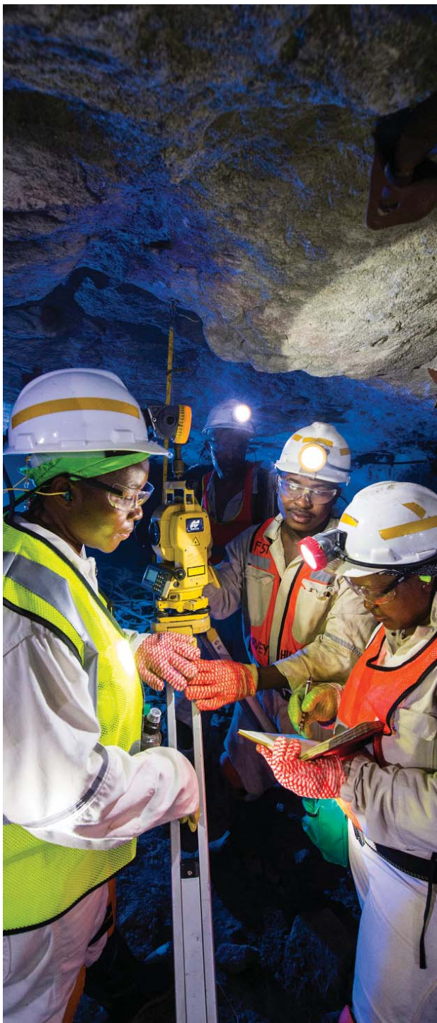
Underground survey in the trackless section, 14 Shaft Impala
