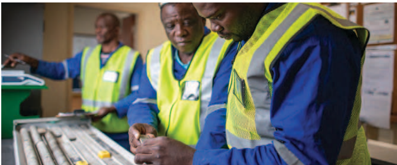
PREPARATION OF SAMPLES FOR ROCK DENSITY MEASUREMENTS, IMPALA
